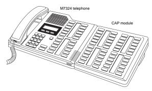
A CAP module is an add-on device that provides 48 extra memory or line buttons. You can connect one or two Norstar CAP modules to the telephone to increase the number of lines it can handle.
